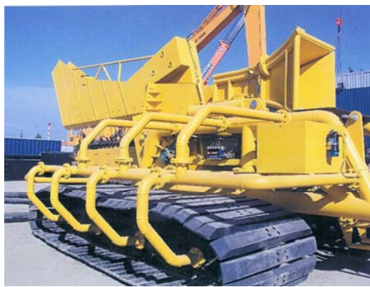
In Simultaneous Lay & Burial Chain Cutter Cable Trenching Mode
